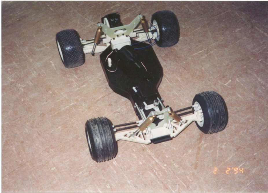
Figure 17. Photograph of RC10 car chassis with modifications to suspension.
